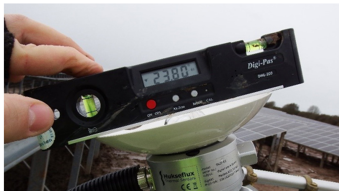
Figure 2: Pyranometer out of inclination
